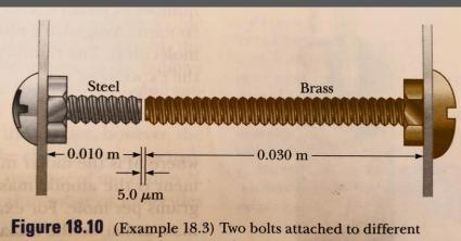
**Figure 18.10** (Example 18.3) Two bolts attached to different parts of an electrical device are almost touching when the temperature is 27°C. As the temperature increases, the ends of the bolts move toward each other.
